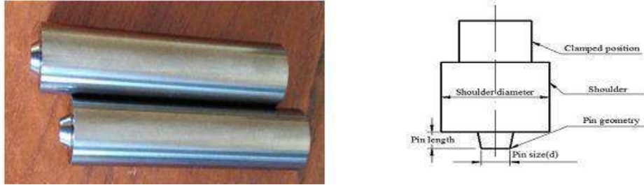
Figure 3. Conical pin tips having 3.4 and 3.8mm length of friction stir spot welding tool.
