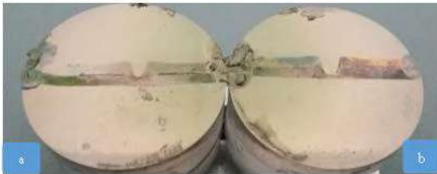
Figure 10. FSSW keyhole cross section metallographic gold coated specimens of AA5754/Ni/AA1050 welded Aluminum alloy sheets a- 3.4mm and b- 3.8mm plunge depths
